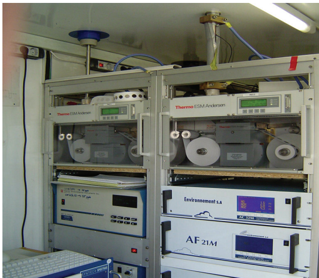
Fig. 7. Instruments of the monitoring station. Measurement program: O_3 , NO , NO_2 , SO_2 , CO , PM_{10} and standard meteorological measurements (temperature, relative humidity, wind speed and direction, global radiation and precipitation)
